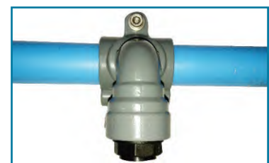
Step 6: Fixing the Droplet on the tube
