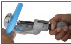
Step 1: Cutting the Tubes
