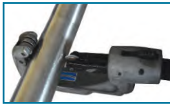
Step 1: Cutting the Tubes
