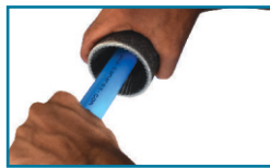
Step 2: Chamfering the Tubes
